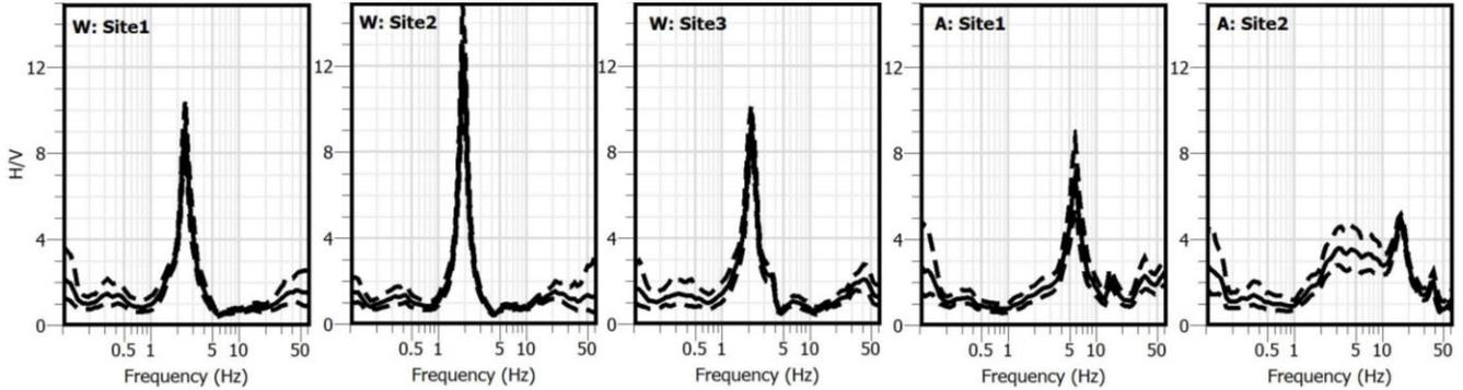
Figure 6. MHVSR curves from the ambient vibration array recordings for each of the five sites.
