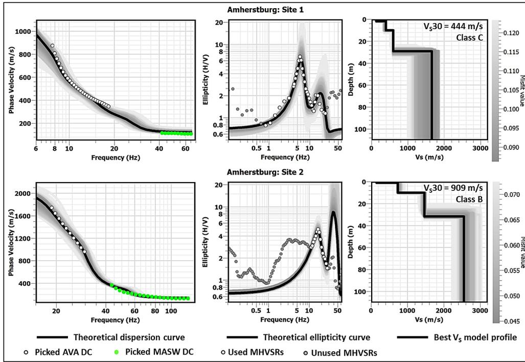
Figure 8. Joint inversion results for the two sites in Amherstburg. Input dispersion and MHVSR data are plotted as circles compared to theoretical dispersion and MHVSR curves (shaded lines) calculated from low misfit  $V_s$  profiles (grey lines) and the minimum misfit  $V_s$  profile (black line).
