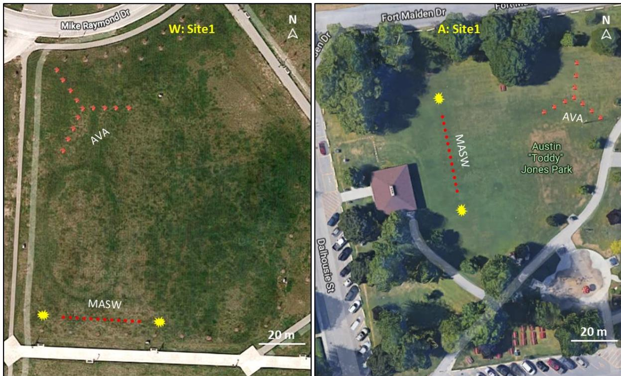
Figure 3. Left panel shows a schematic of the AVA and MASW array data collection for Windsor site 1, and right panel shows the same for Amherstburg site 1.
