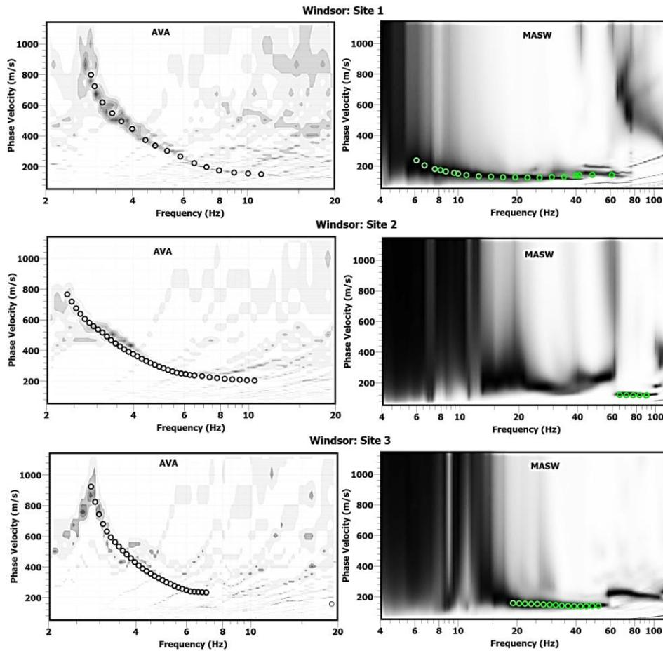
Figure 4. MSPAC-processed dispersion histograms from AVA recordings (left panels) and f-k-processed dispersion histograms from MASW recordings (right panels) generated for the three sites in Windsor. Open circles show manually picked dispersion estimates.
