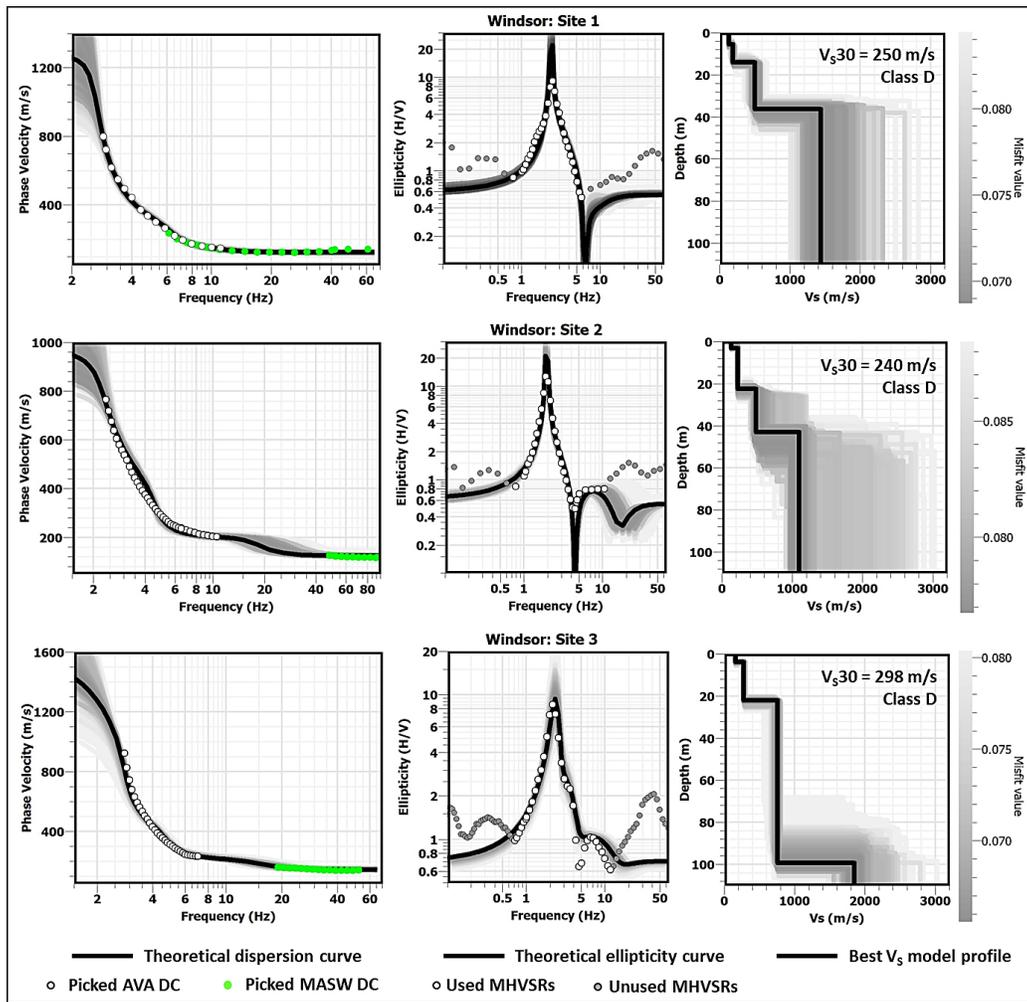
Figure 7. Joint inversion results for the three sites in Windsor. Input dispersion and MHVSR data are plotted as circles compared to theoretical dispersion and MHVSR curves (shaded lines) calculated from low misfit  $V_s$  profiles (grey lines) and the minimum misfit  $V_s$  profile (black line).
